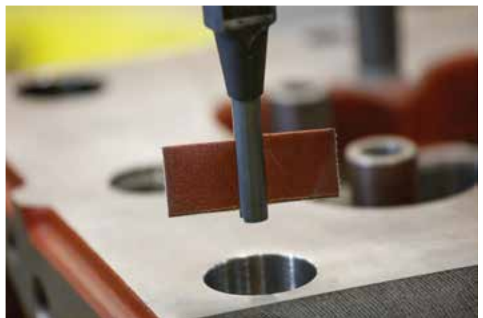
Emery cloth spins between the hard metal fingers, removing the burrs and finishing the edges.
